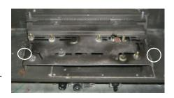
Remove the 10 screws holding the Access Panel in place.
